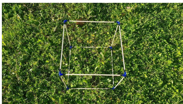
Figure 2. Example of a biocube, captured during Spring, in Santarém, Portugal. The cube structure has edges measuring 30 cm in length.
